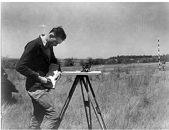
Figure 3: Chain and compass for surveying (above) and plane tables (below) – very common through until late 1960's
