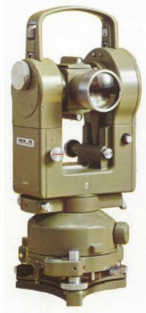
Figure 5: Wild T2 Universal Theodolite (Pictures from the Archive of the Wild Heerbrugg AG, apart from the tape which was found from general Internet search)
